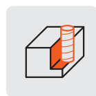
Fresatura laterale e frontale Side and face milling
